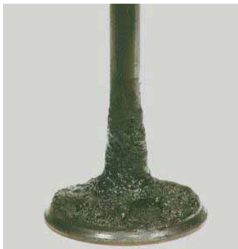
Picture D - Intake valve before P.i. treatment
