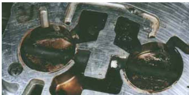
Picture J - Carburetor plates before P.i. treatment
