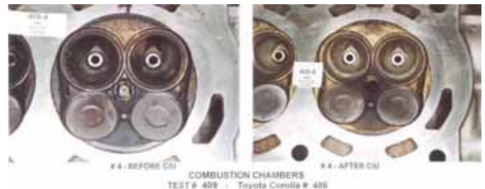
Picture F - Combustion chamber before P.i. treatment
